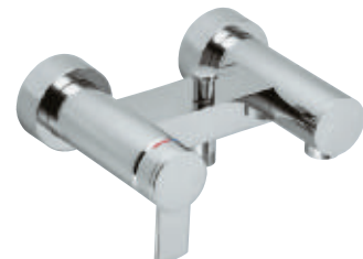
54920 Single lever bath tub mixer exposed, ceramic cartridge with temperature limiter, with automatic return bath tub/shower
