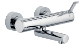
54921 Single lever basin mixer exposed, ceramic cartridge with temperature limiter Projection: 150 mm, 200 mm, 250 mm
