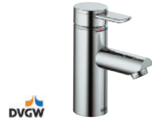
DVGW 54904 Single lever basin mixer without pop-up waste, middle size model, 1-hole installation, ceramic cartridge with temperature limiter
