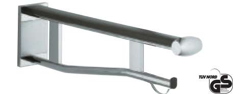
34905 Pivoted supporting rail for WC* firmly fastened, with synthetic covered support and removable toilet paper holder with rollbrake Projection: 700/850 mm
